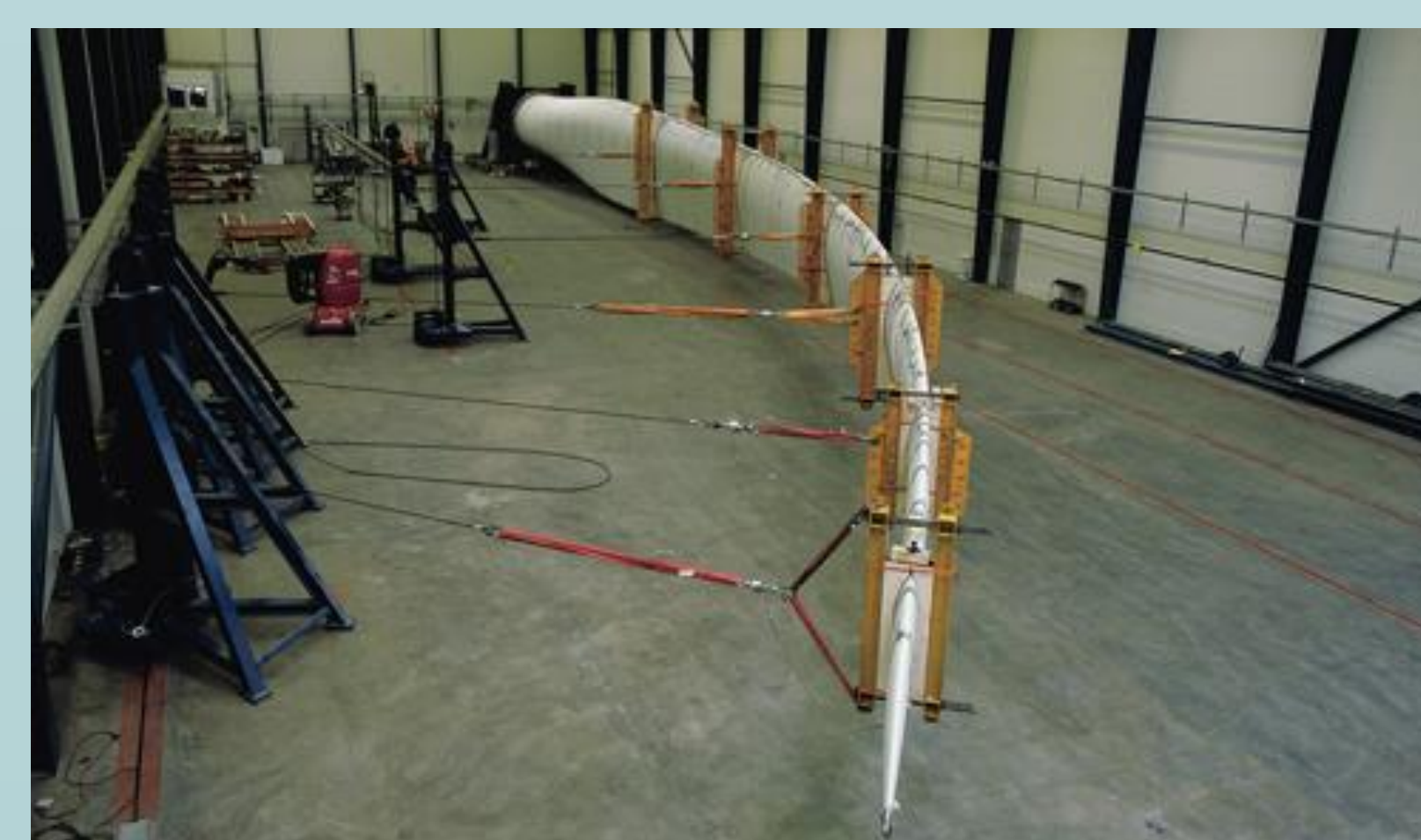
Fig 3. The large bending deformation experienced by a wind turbine blade during a structural test.
